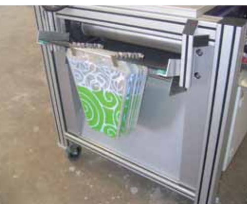
INPUT UNIT: INPUT OF THE SLEEVES READY FOR LABELING
