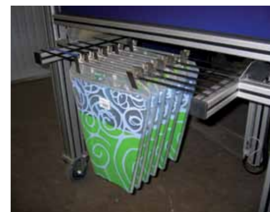
OUTPUT UNIT: SLEEVES ALREADY LABELED
