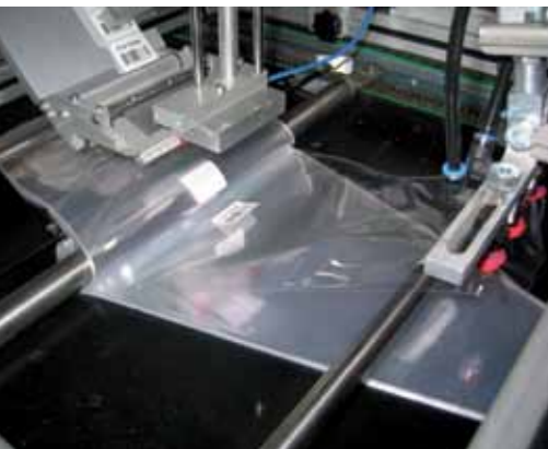
THE LABEL UNIT: THE ADVANCED LABEL HEAD ENSURES PRECISE LABEL POSITIONING
